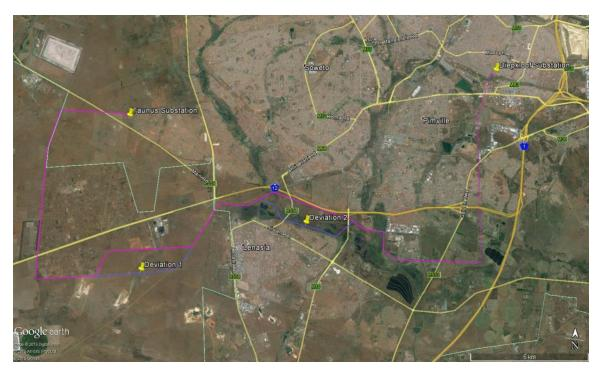
**Figure 1:** Proposed alignments for Taunus – Diepkloof 132kV. The purple line represents the proposed alignment and the blue sections the alternative alignments.
